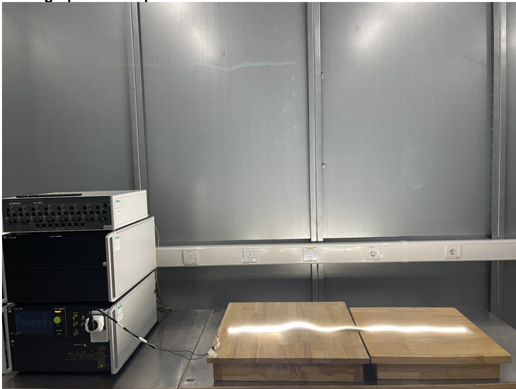
Photograph 6: Set-up for EFT on DC Power Port
