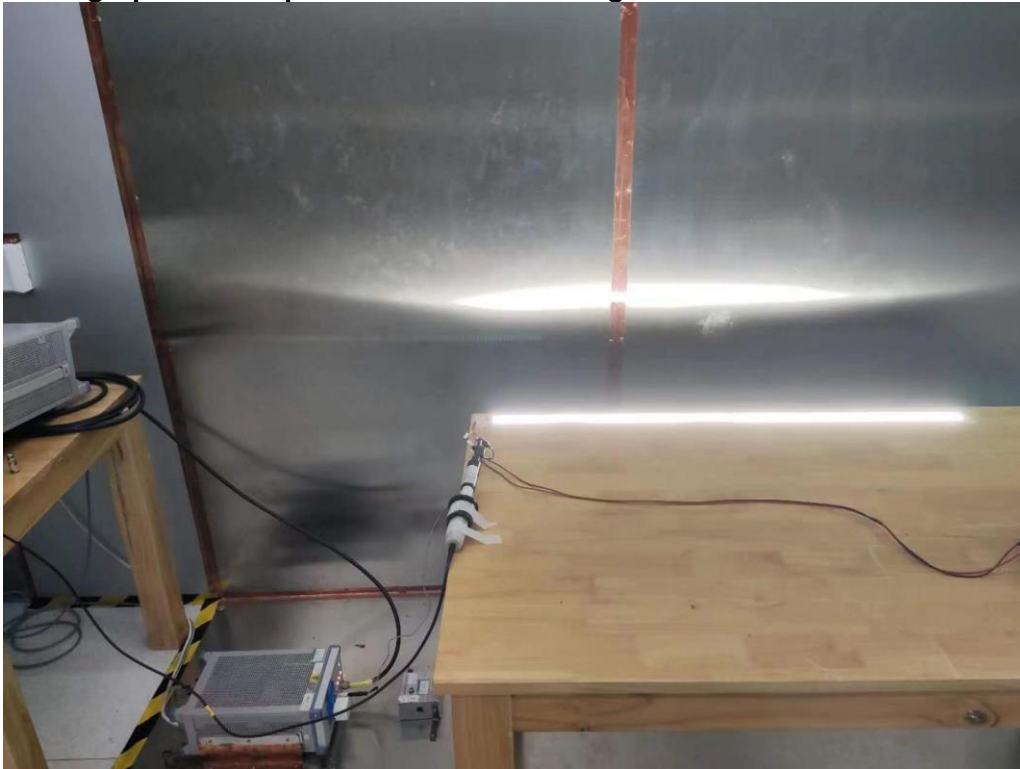
Photograph 4: Set-up for Injected Currents on DC Power Port (CS)
