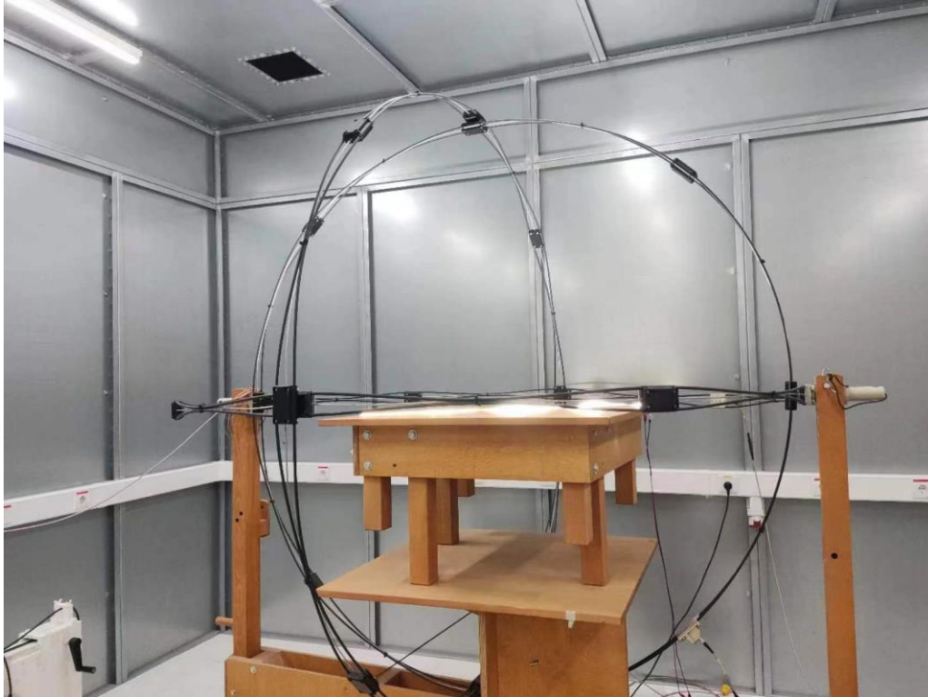
Photograph 2: Set-up for Radiated Electromagnetic Disturbances (30MHz-1000MHz)
