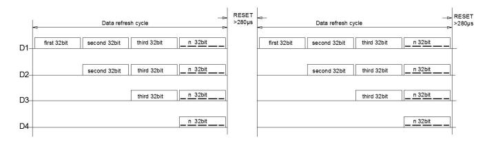
PS. D1 is the data sent by MCU port, D2, D3, D4 are data shaped and transmitted by cascade circuit.
