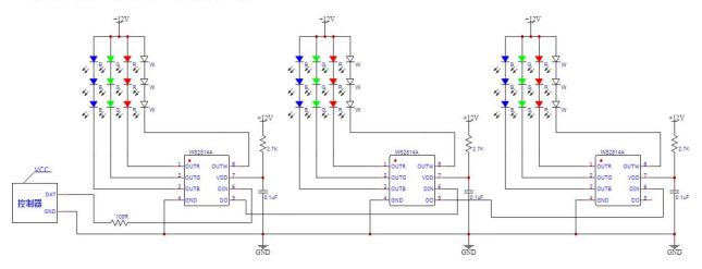
3.24V供电应用参考电路(每通道带6颗LED):24V power supply application reference circuit (each channel with 6 LED):
