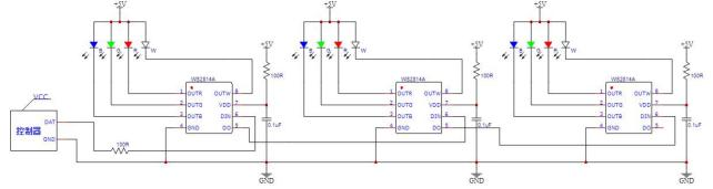
2.12V供电应用参考电路(每通道带3颗LED): 12V power supply application reference circuit (each channel with 3 LED):
