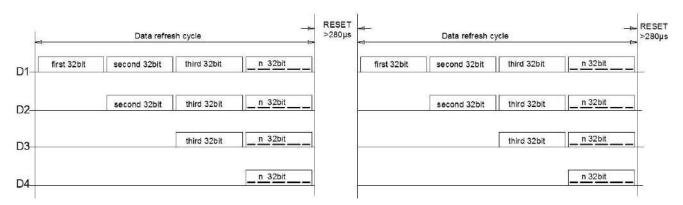
Note: The data of D1 is send by MCU, and D2, D3, D4 through IC internal reshaping amplification to transmit.
