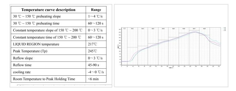
Remarks:All temperatures referred are measured on the surface of the package body.
