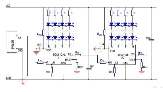
3. Reverse polarity application - external constant current driver IC (UCS512H4)
