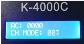
5. Press "MODE" again to enter "AC" test mode and the lamps automatically light up; the controller displays as shown in the following figure (when the interval channel is address writing, the setting cannot be adjusted)
