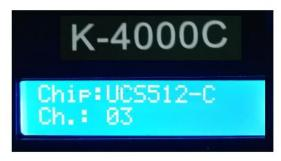
8. After writing the address, first press "CHIP" and then "MODE" to switch to the play mode, and switch the chip to Chip: 10. At this time, it is DMX512 standard protocol and 250K play mode. You can press the "MODE" and "SPEED" keys to switch the play mode
