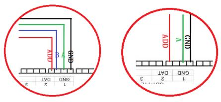
Note: For the installation of some DMX512 lamps, the controller output ports do not need to connect with the ADDR
