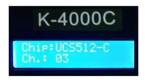
2. Press "CHIP" to switch the DMX512 IC model, and "SPEED+"/"SPEED-" to adjust the interval channels, as shown in the following figure:
