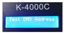
2. After about 2s, the controller will enter the lamp address testing interface as shown in the figure below:
