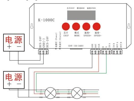
Like the above diagram, wired the line and start the controller, press "CHIP" and "MODE" at the same time switch to coding mode, adjust to Chip: 61 that is UCS512A or B coding mode, as below:
