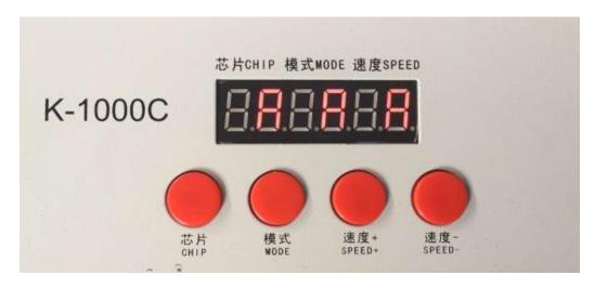
3. After finished address code, press "CHIP" first and at the same time press "MODE"button, switch to playback mode, switch the chip to Chip: 10, this is the DMX512 standard agreement 250Kbps playback mode. At this time, press MODE button and SPEED button can separately switch playback mode and adjust speed, as below:
