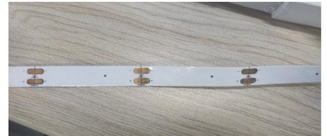
5. Results: After 30 days of chlorine-proof accelerated test, the electric performance of the strip is normal, the appearance has no obvious change, and there is no water or corrosion phenomenon at the outlet end of the
