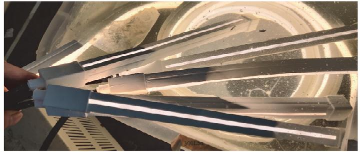
Changes: The electric performance of the strip is normal, and the surface is unchanged.
