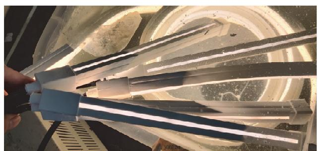
Changes: The electric performance of the strip is normal, and the surface is unchanged.
