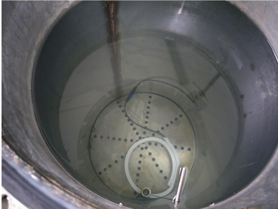
Photo 3: IPX8 test of model NP-T1615-W40-10-CC
