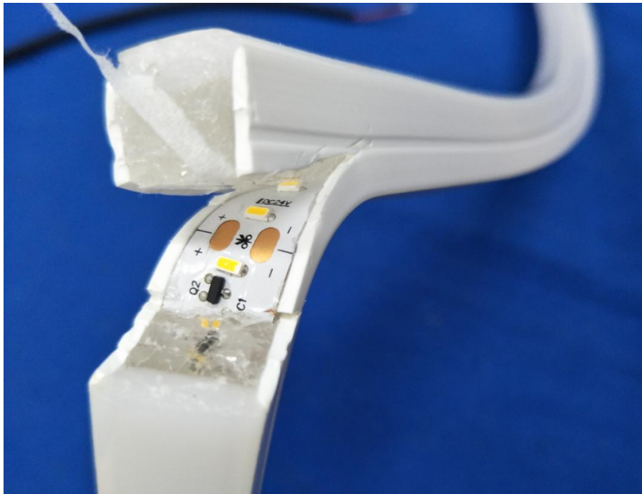
Photo 4: After IP6X and IPX8 test of model NP-T1615-W40-10-CC
