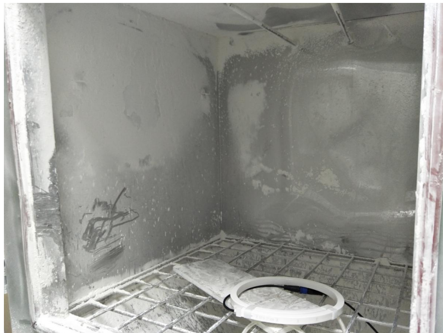
Photo 2: IP6X test of model NP-T1615-W40-10-CC
