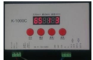
4 Press the "MODE" button to start addressing the led strip, the controller shows "AAA", as shown below:
