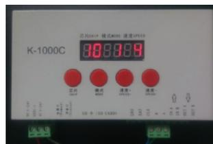
7 The display of the first and second digits of the controller must be "10". If it is other numbers, the led strip cannot be controlled normally. Adjust the "CHIP" button to select the displayed values of these two digits.
