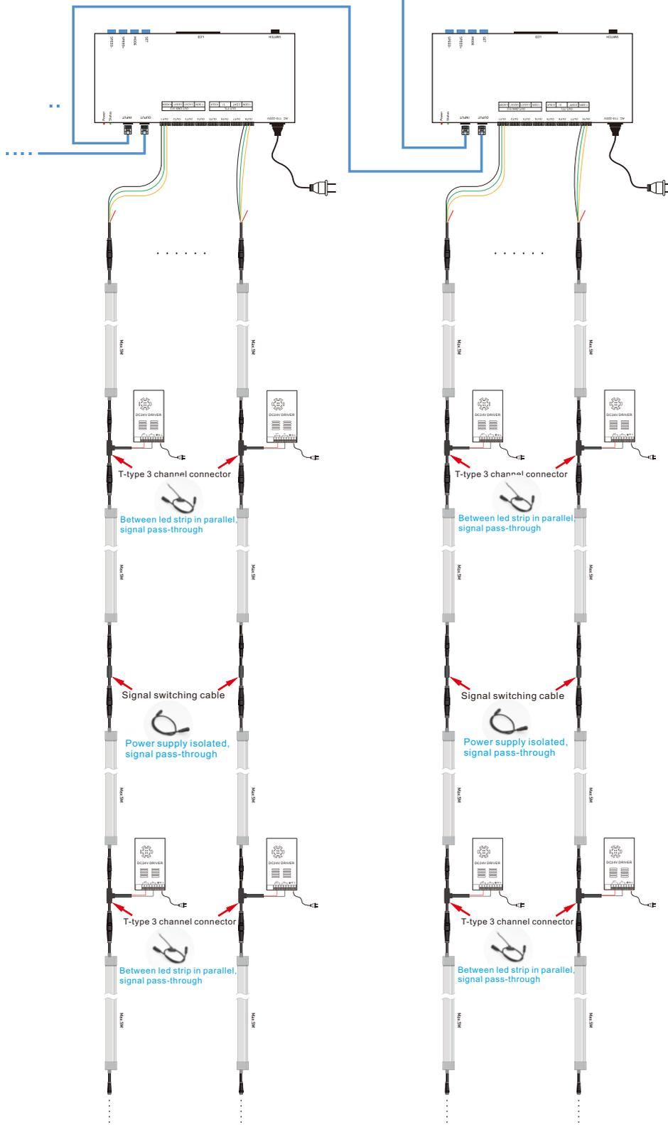
After the led strip is connected to the signal wire and power supply wire correctly, it is necessary to use a special addresser to address the led strip, then the controller / console can run the control effect program.
