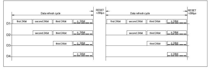
Note: D1 is the data from MCU, and D2, D3, D4 are from Cascade Circuits.
