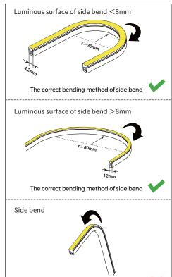
The wrong bending method of side bend
