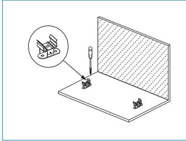
Remove the light, aluminum profile and rotating brackets from the box, and fix the rotating brackets to the needed position with a screwdriver.
