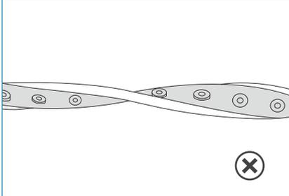
Do not twist the LED wall washer during the installation process.
