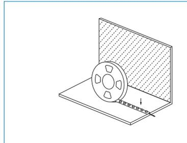
Install the product where you need it (ensure the wall is smooth), refer to the installation distance diagram for the specific glowing effect, and stick it firmly.
