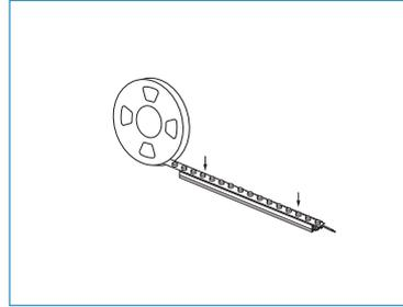
Put the light into the aluminum profile, and press the light down along the profile to ensure the light is tightly stuck into it. Then fasten the profile on the rotating brackets (according to the glowing angle requirements, the rotating bracket can be adjusted).
