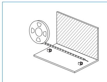
Take the light out of the box, then put the light into the clips and secured it (refer to the installation distance diagram for the specific glowing effect).
