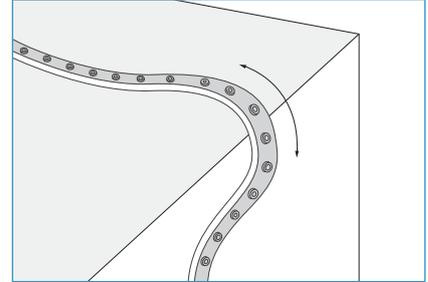
When LED wall washer meets the corner during the installation process, the LED wall washer must be kept facing up and the back facing down, maintaining a certain bending arc,  $\Phi \geq 150\text{mm}$ .
