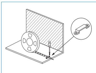
Place the light where needed, and refer to the installation distance diagram for the specific glowing effect.
