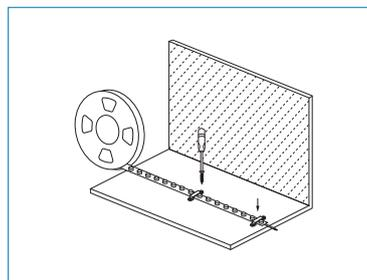
Remove the silicone mounting clips and screws from the package box, and fix these clips with a screwdriver.
