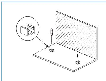
Remove the stainless steel mounting clips and screws from the packing box, and use a screwdriver to install these clips where needed.
