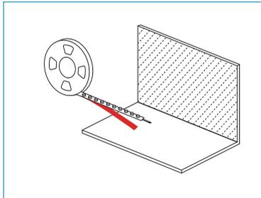
Remove the product from the packaging box and tear off the tape on the back.
