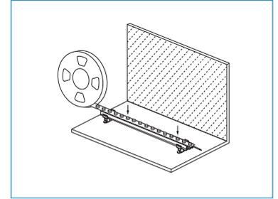
The specific glowing effect can be adjusted according to the needs of the application. After the installation, connect the light to the low-voltage driver and energize it.
