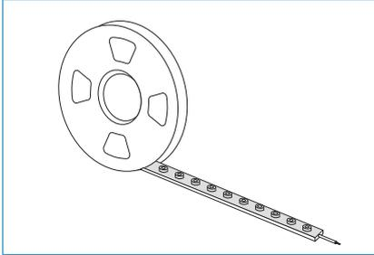
During the installation process, the LED wall washer is taken out from the reel naturally and keep it as straight as possible.
