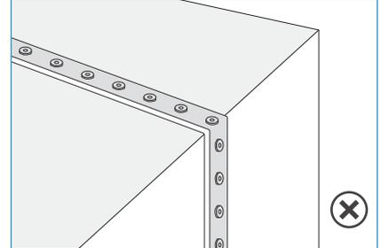
When the LED wall washer meets the corner during the installation process, the LED wall washer must be kept facing up and the back down, and it cannot be bent at right angles.
