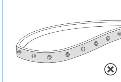
Do not fold the LED wall washer in half or bend it at a small angle during the installation.
